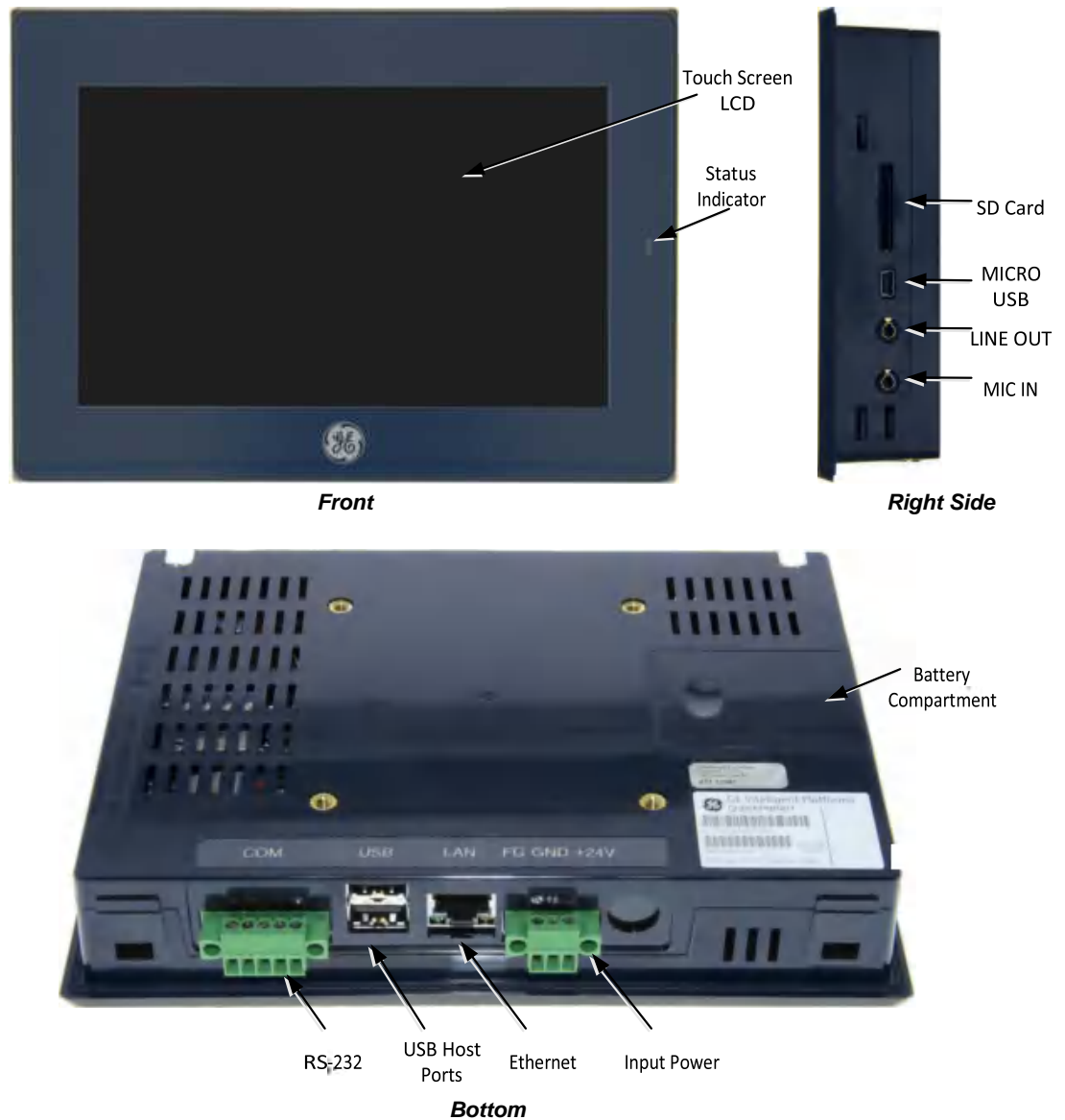
Figure 1. QuickPanel+ Hardware Features
